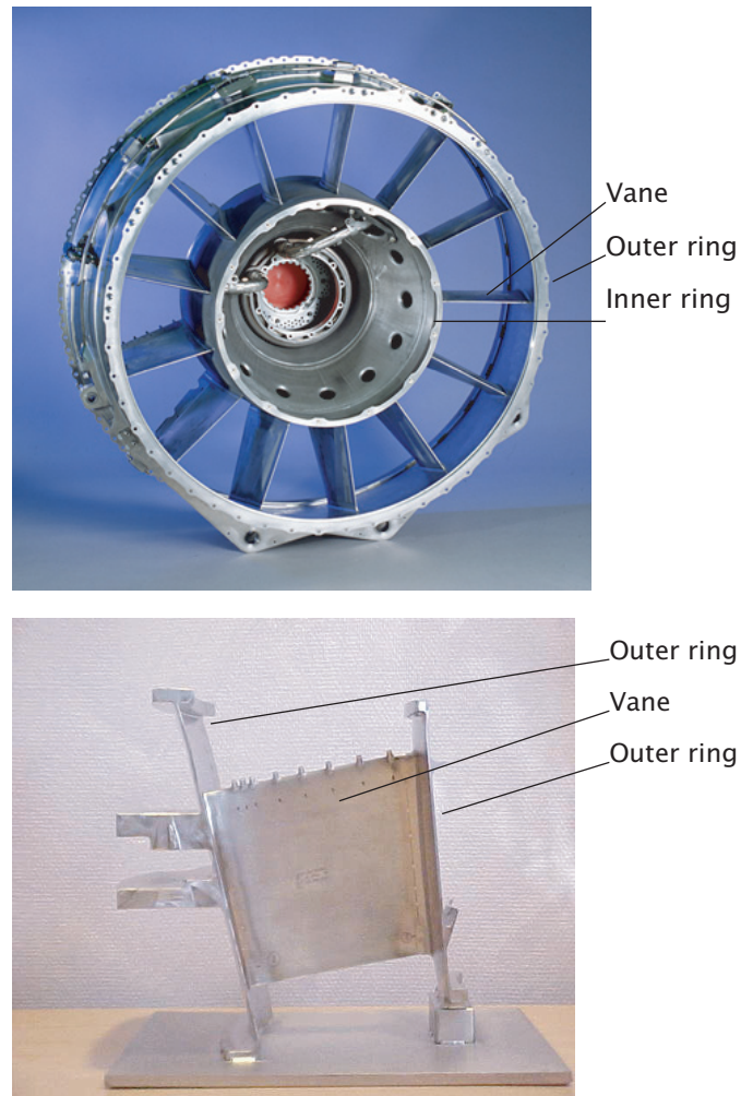
Figure 2: a) Turbine component consisting of an inner- and an outer ring and 13 vanes. b) experimental component (1/13 of the turbine component).
