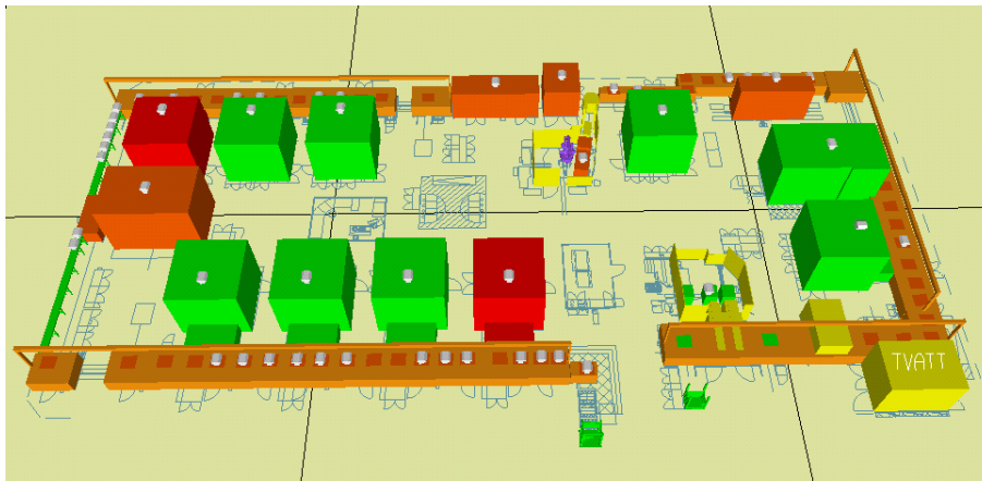
Figure 2: DES layout of the case study. The operation modes of the machines are indicated by the different colours; green for busy, yellow for idle, red for failure, and orange for blocked.
