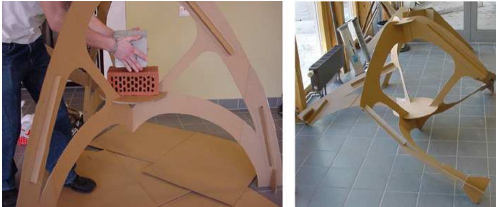
FIG. 4 - Loading of the structure (left) and the structure as it appeared following failure (right).
