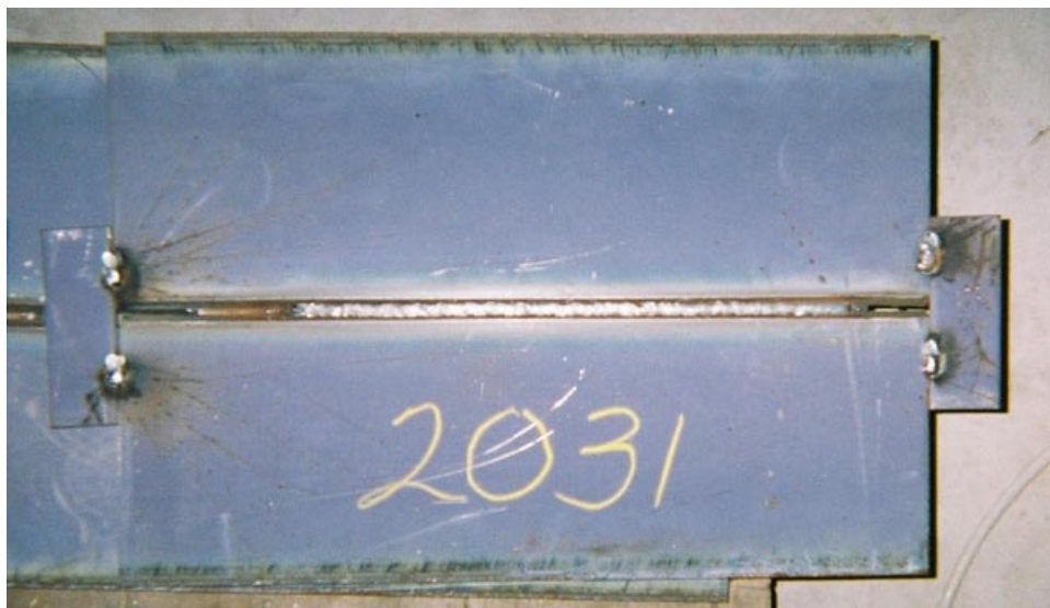
Figure 19: Example of V-groove weld. These workpieces are single sided and the seams have to be covered from the back by ceramic material to prevent welding flux from passing through the seams, and thereby cause low welding quality.
