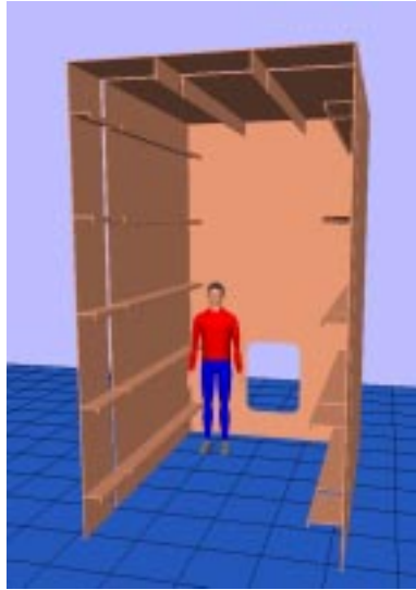
Figure 2: A double hull-cell in ROWER-2 with man-hole through which the robot equipment is manually transported. One of the walls and the floor have been excluded from the picture.
