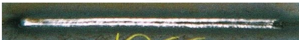
Figure 21: Pictures of some selected fillet welds.
